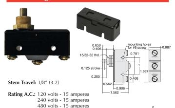
Mounting: #15/32-32 thread; nut and lockwashers furnished, also two 0.140" dia. mounting holes in body
